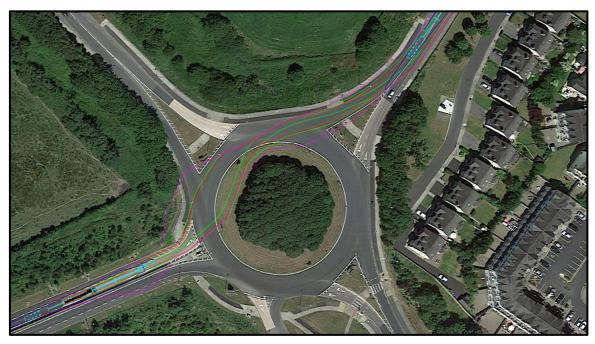
Figure 41: Clonmacken Roundabout – WTG blade deliveries arriving from the west – swept path
