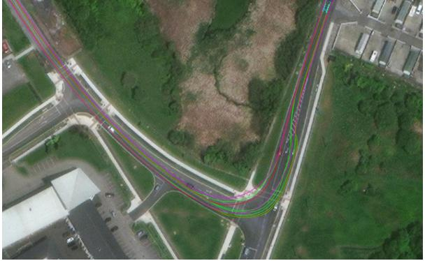
Figure 39: Junction of R464 and Knockalisheen Road – Oversized tower section – swept path
