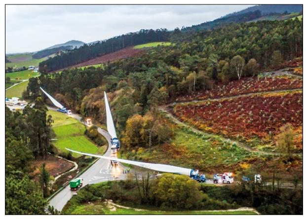
Figure 3: Blade lifter trailers in convoy transitioning from tilted to lowered to avoid overhead line
