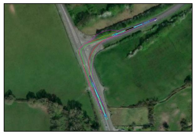
Figure 11: Junction of Foynes Port Road with the N69 - swept path
