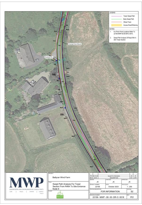
Figure 77: Area No. 9 - Tower section delivery—swept path
