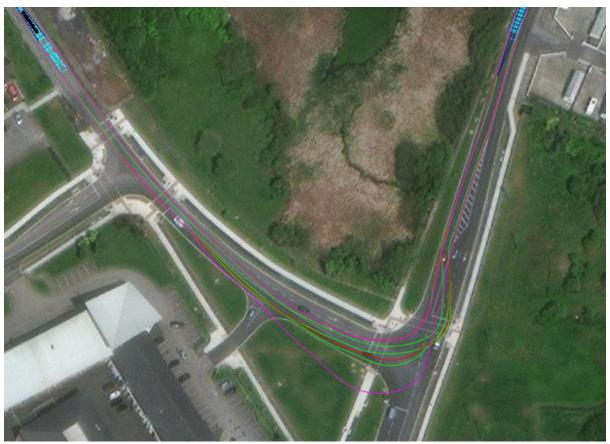
Figure 38: Junction of R464 and Knockalisheen Road –Blade Lifter trailer with blade inclined at 60° - swept path
