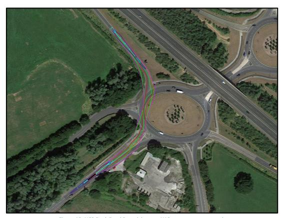
Figure 18: N69 Dock Road Roundabout to N18 on-ramp – swept path
