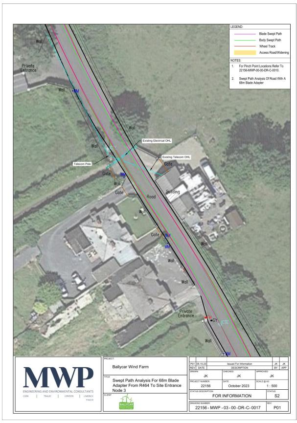
Figure 57: Area No. 3 – Blade Lifter trailer with blade raised to 60° - swept path
