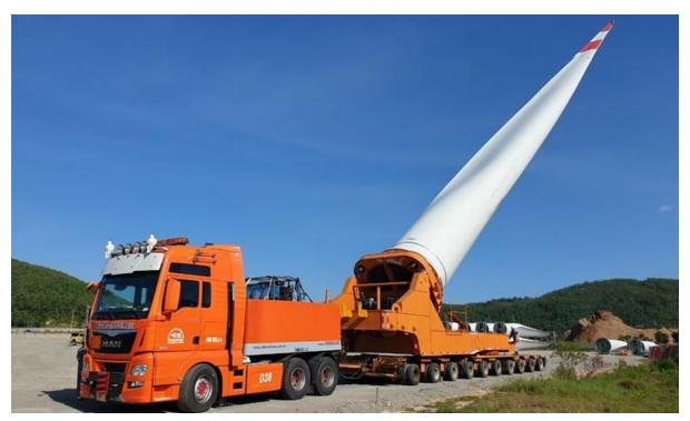
Figure 2: Blade lifter trailer with blade tilted to  $60^{\circ}$  to the horizontal
