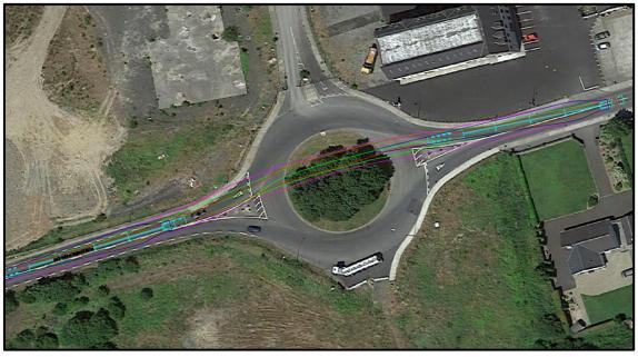
Figure 15: Clarina Roundabout swept path through central island
