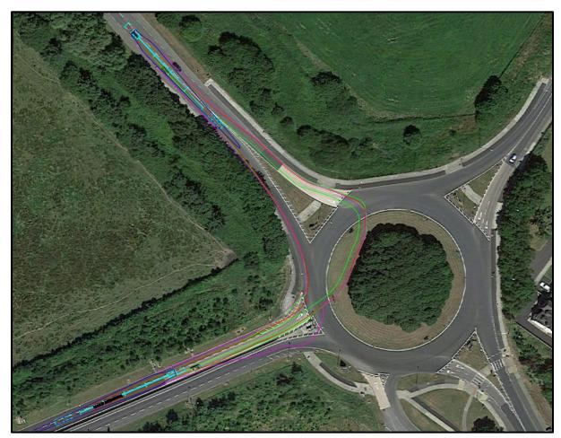
Figure 29: Clonmacken Roundabout – swept path
