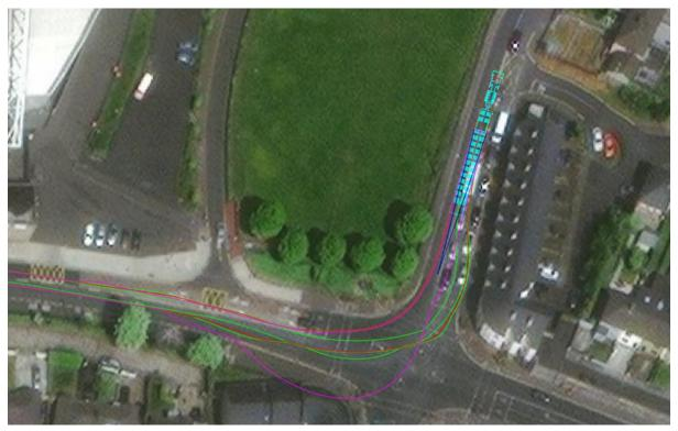
Figure 48: Cratloe / Kileely Road junction - Blade lifter with blade raised to 60° - swept path
