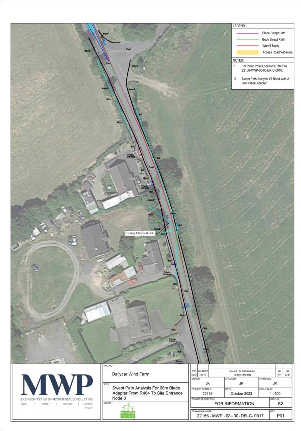
Figure 73: Area No. 8 – Blade Lifter with blade raised to  $60^{\circ}$  – swept path
