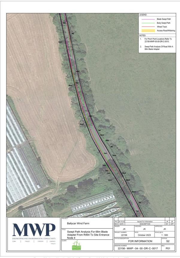
Figure 59: Area No. 4 – Blade Lifter trailer with blade raised to 60° - swept path
