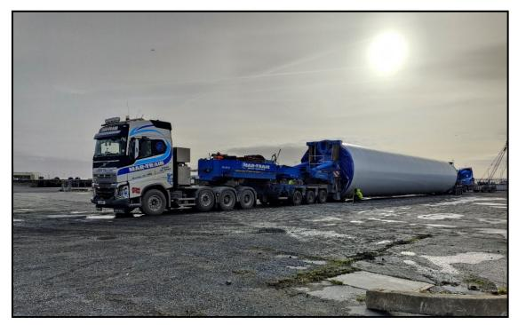
Figure 6: Bogie type tower transporter
